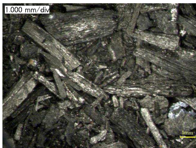
Fig. 2 Microscopic (25 times enlarged) view of wooden charcoal
